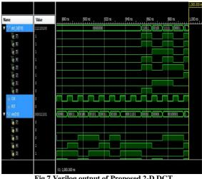
Fig.7 Verilog output of Proposed 2-D DCT
