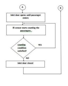
First we have to generate a ticket through app, then that ticket is scanned while boarding the bus. Bus in turns check for the number of passenger if bus contains more number of passenger, then it displays "wait for the next bus". Once barcode is scanned processor check for the validity, if it is valid then door opens for passenger service and IR sensor helping for counting the number of passengers boarded. If ticket is invalid then door will remain closed and buzzer gets activated.
