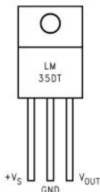
Fig.3 Temperature Sensor LM35
