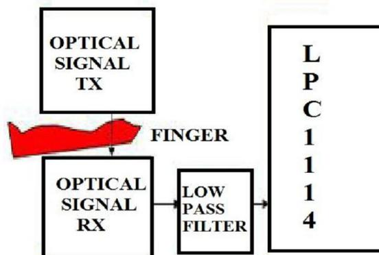
Fig. 5 Circuit Diagram of Heart Beat Sensor
