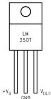
Fig.3 Temperature Sensor LM35
