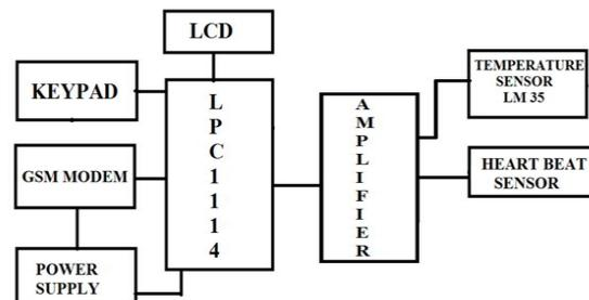
Fig.1 Block Diagram of Health Monitoring System
