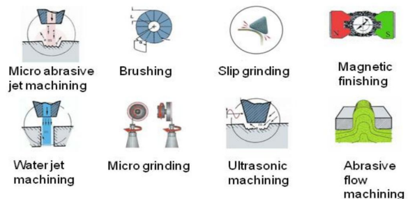
Fig. 3: Mechanical preparation processes
