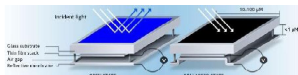
Figure 1: Core of an IMOD Display
