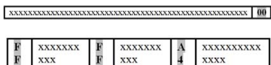
Fig.3. COBS code blocks. Each COBS code block begins with a single code byte (shown shaded), followed by zero or more data bytes.
