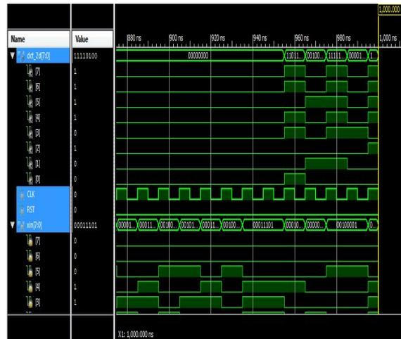
Fig.7 Verilog output of Proposed 2-D DCT
