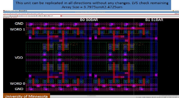
Figure 14: 4 cell layout for 6T SRAM that can be mirrored in all the directions
