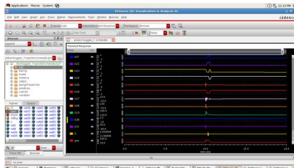
Figure 10: Simulation Result of 32-bit KS Adder
