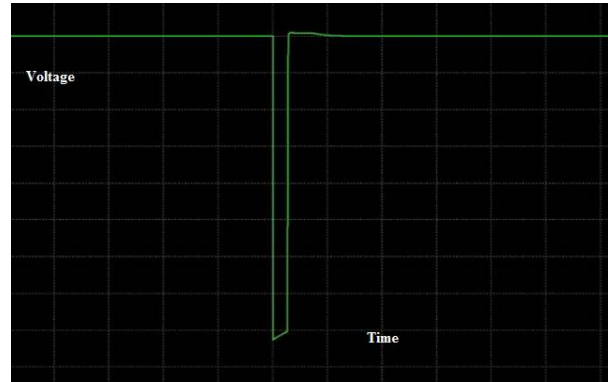
Fig.9 Simulated Pulser output signal on LT Spice simulator
