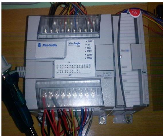
Figure 1. MicroLogix 1200 By Allen-Bradley which is a 24 point controller
