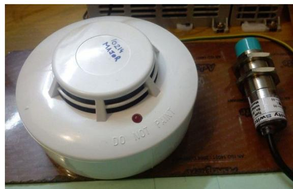
Figure 2. Digital Smoke Sensor alongside with Proximity Sensor (right)
