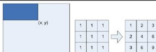
Figure 4. Integral Image generation. It shows a 3x3 image and its integral image representation
